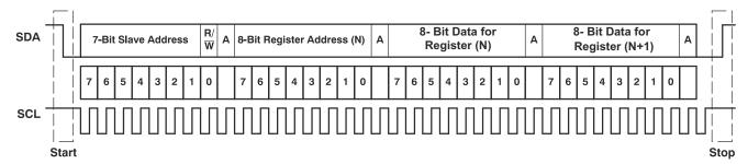
Figure 8-66. Typical I<sup>2</sup>C Sequence
