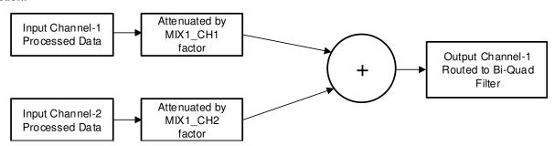
Figure 8-18. Programmable Digital Mixer Block Diagram
