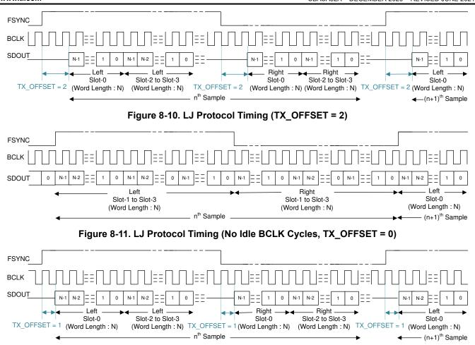
Figure 8-12. LJ Protocol Timing (TX OFFSET = 1 and BCLK POL = 1)
