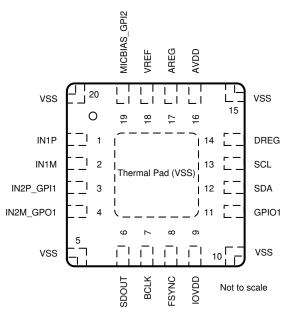
Figure 6-1. RTE Package, 20-Pin WQFN With Exposed Thermal Pad, Top View
