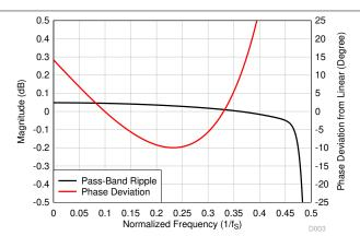
Figure 8-50. Ultra-Low-Latency Decimation Filter Pass-Band Ripple and Phase Deviation
