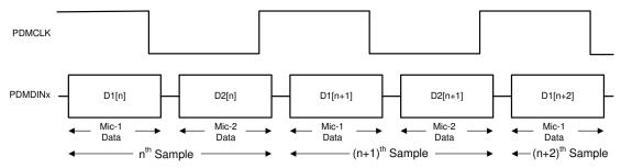
Figure 8-65. Digital PDM Microphone Protocol Timing Diagram
