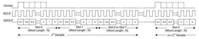
Figure 8-4. TDM Mode Protocol Timing (TX\_OFFSET = 0 and BCLK\_POL = 1)
