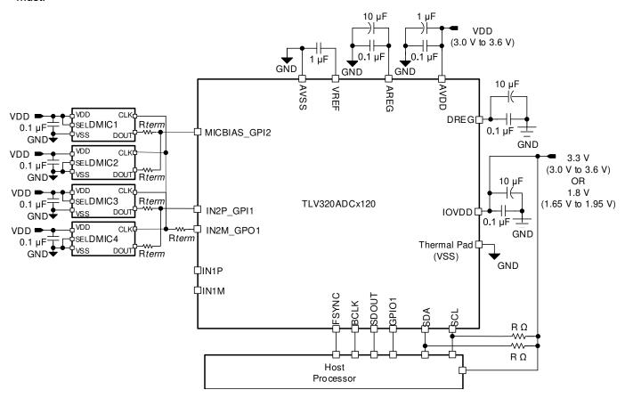
Figure 9-6. Four-Channel Digital PDM Microphone Recording Diagram
