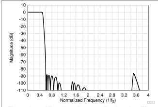
Figure 8-55. Ultra-Low-Latency Decimation Filter **Magnitude Response**
