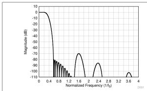
Figure 8-33. Linear Phase Decimation Filter Magnitude Response
