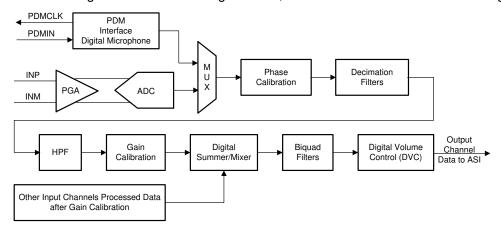
Figure 8-16. Signal-Chain Processing Flowchart
