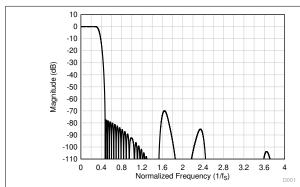
Figure 8-31. Linear Phase Decimation Filter Magnitude Response
