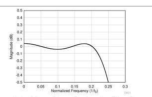
Figure 8-34. Linear Phase Decimation Filter Pass-Band Ripple
