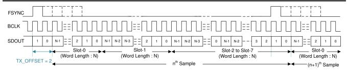
Figure 8-3. TDM Mode Protocol Timing (No Idle BCLK Cycles, TX\_OFFSET = 2)
