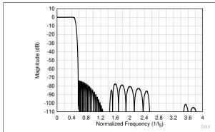
Figure 8-25. Linear Phase Decimation Filter Magnitude Response
