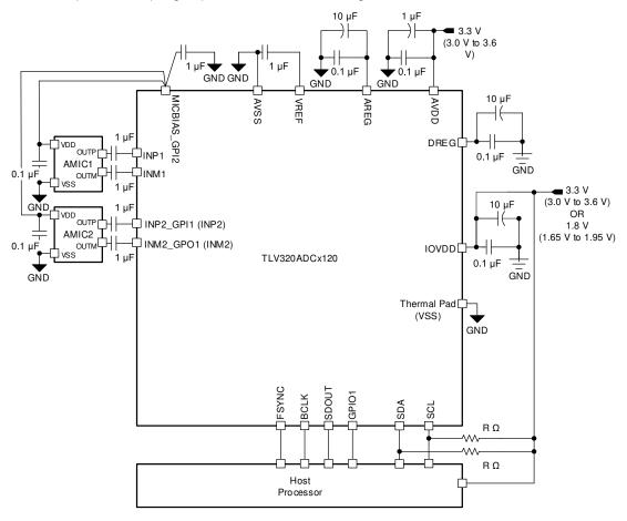
Figure 9-1. Two-Channel Analog Microphone Recording Diagram
