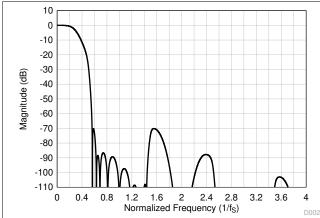
Figure 8-61. Ultra-Low-Latency Decimation Filter Magnitude Response
