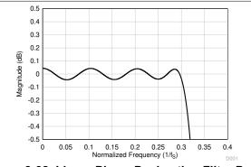
Figure 8-32. Linear Phase Decimation Filter Pass-Band Ripple
