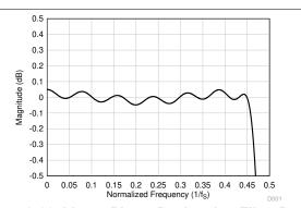
Figure 8-30. Linear Phase Decimation Filter Pass-Band Ripple
