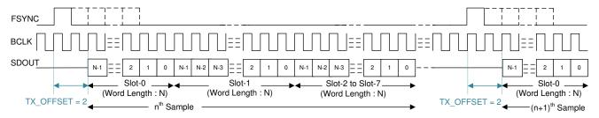
Figure 8-2. TDM Mode Protocol Timing (TX\_OFFSET = 2)
