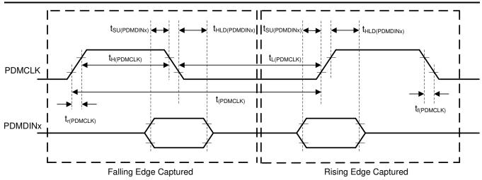
Figure 7-3. PDM Digital Microphone Interface Timing Diagram
