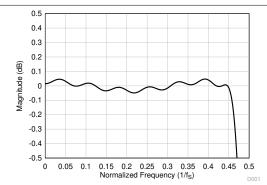
Figure 8-28. Linear Phase Decimation Filter Pass-Band Ripple
