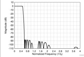
Figure 8-51. Ultra-Low-Latency Decimation Filter Magnitude Response
