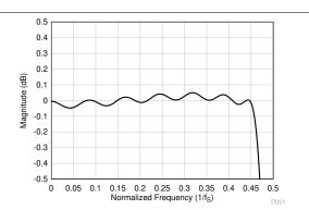
Figure 8-22. Linear Phase Decimation Filter Pass-Band Ripple
