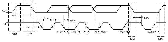
Figure 7-1. I<sup>2</sup>C Interface Timing Diagram
