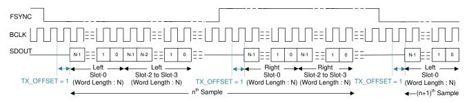
Figure 8-6. I<sup>2</sup>S Protocol Timing (TX\_OFFSET = 1)
