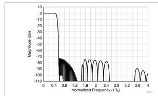
Figure 8-19. Linear Phase Decimation Filter Magnitude Response
