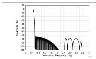
Figure 8-21. Linear Phase Decimation Filter Magnitude Response
