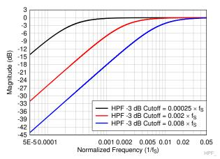
Figure 8-17. HPF Filter Frequency Response Plot
