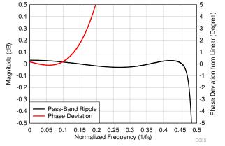
Figure 8-59. Ultra-Low-Latency Decimation Filter Magnitude Response
