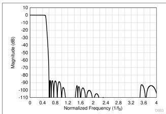
Figure 8-49. Ultra-Low-Latency Decimation Filter Magnitude Response
