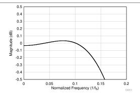
Figure 8-36. Linear Phase Decimation Filter Pass-Band Ripple
