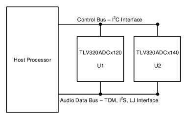
Figure 8-13. Multiple Devices With Shared Control and Audio Data Buses
