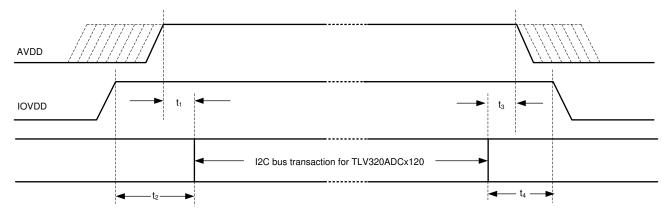
Figure 10-1. Power-Supply Sequencing Requirement Timing Diagram
