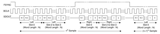
Figure 8-5. I<sup>2</sup>S Mode Standard Protocol Timing (TX OFFSET = 0)
