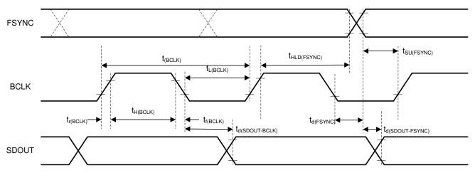
Figure 7-2. TDM (With BCLK\_POL = 1), I<sup>2</sup>S, and LJ Interface Timing Diagram
