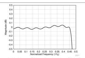
Figure 8-26. Linear Phase Decimation Filter Pass-Band Ripple
