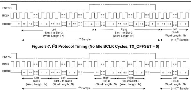
Figure 8-8. I<sup>2</sup>S Protocol Timing (TX\_OFFSET = 0 and BCLK\_POL = 1)
