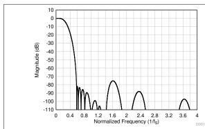
Figure 8-35. Linear Phase Decimation Filter
