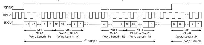
Figure 8-9. LJ Mode Standard Protocol Timing (TX\_OFFSET = 0)
