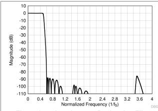
Figure 8-47. Low-Latency Decimation Filter Magnitude Response
