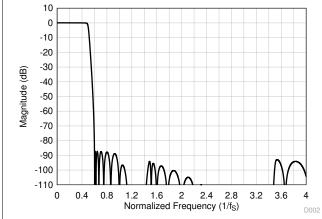
Figure 8-37. Low-Latency Decimation Filter Magnitude Response
