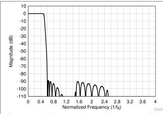
Figure 8-53. Ultra-Low-Latency Decimation Filter Magnitude Response
