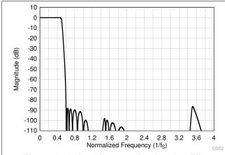
Figure 8-43. Low-Latency Decimation Filter Magnitude Response
