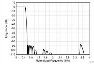
Figure 8-45. Low-Latency Decimation Filter Magnitude Response
