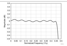
Figure 8-20. Linear Phase Decimation Filter Pass-Band Ripple
