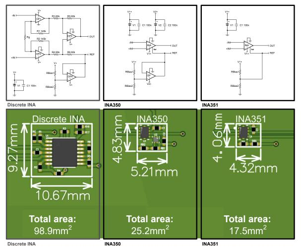
Figure 2. PCB Layout Comparison of Three Designs
