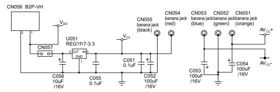
Figure 3-2. DEM-DAI/DAC Connector and Regulator Schematic
