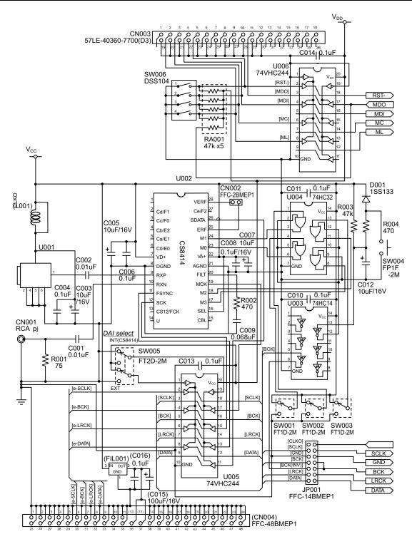
Figure 3-3. DEM-DAI/DAC Digital Audio Interface Schematic
