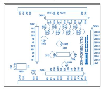
Figure 3-8. DEM-PCM1780/81/82 Board Layout—Silkscreen
