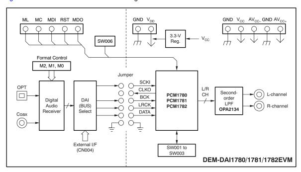
Figure 1-1. DEM-PCM1780/81/82 EVM Functional Block Diagram
