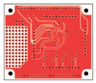
Figure 3-10. DEM-PCM1780/81/82 Board Layout—Bottom View
