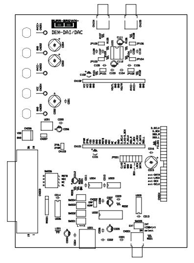
Figure 3-5. DEM-DAI/DAC Board Layout—Silkscreen
