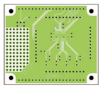
Figure 3-9. DEM-PCM1780/81/82 Board Layout—Top (Component) Side
