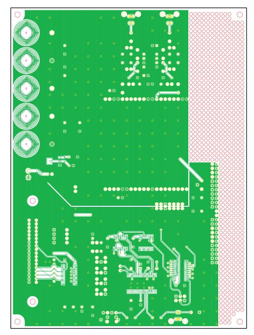
Figure 3-6. DEM-DAI/DAC Board Layout—Top (Component) Side
