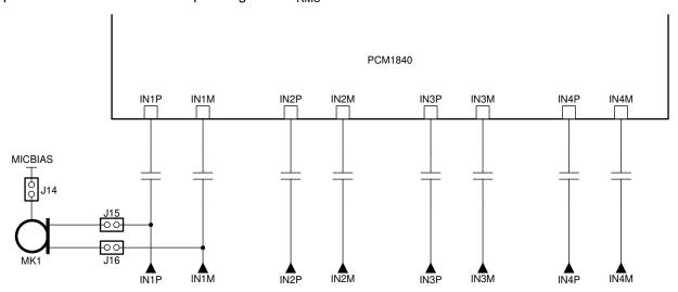
Figure 3-1. PCM1840EVM Input Architecture
