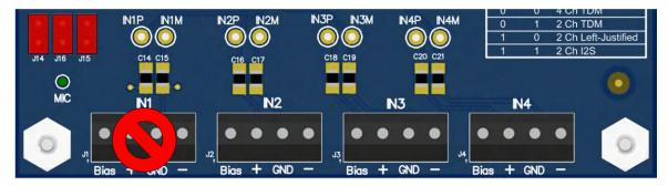
Figure 3-3. PCM1840EVM Connection for the Onboard Microphone Test
