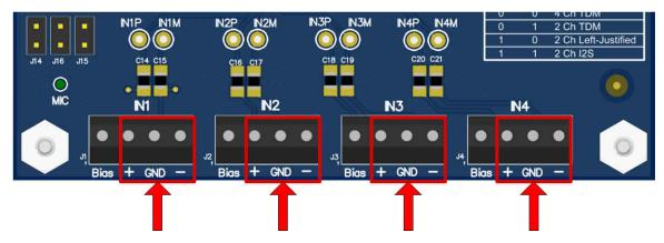
Figure 3-2. PCM1840EVM Connection for Line Input Application
