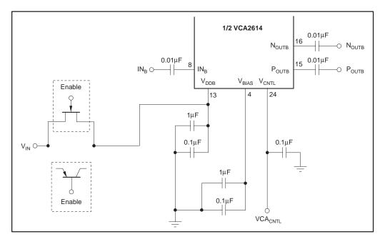
Figure 5. Example Transistor Connection to the VCA261x
