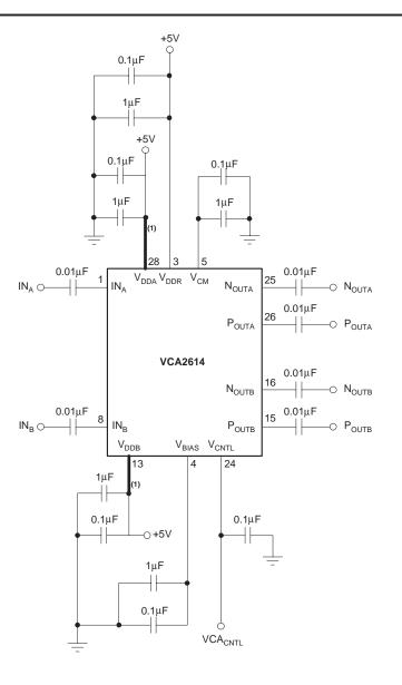
NOTE: (1) When powering down a single channel, one or the other supply pins (V\_DD\chi) must be disconnected.
