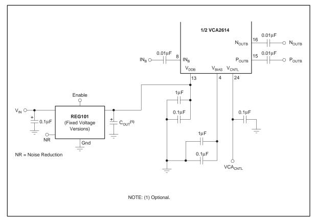
Figure 3. Example LDO Connection to the VCA261x
