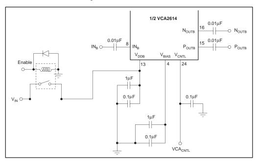
Figure 4. Example Relay Connection to the VCA261x
