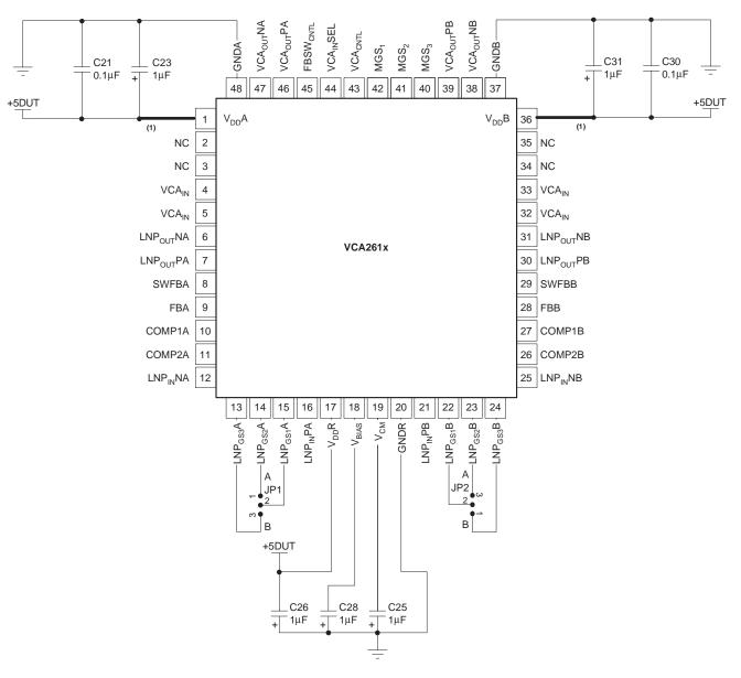
NOTE: (1) When powering down a single channel, one or the other supply pins ( $V_{DDX}$ ) must be disconnected.
