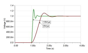
Figure 3. Slew Rate Comparison
