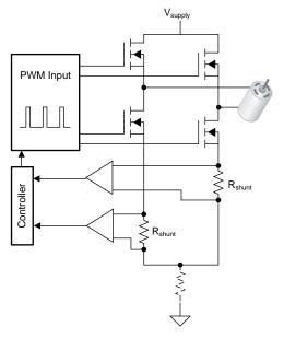
Figure 1. H-Bridge Motor Driver with Low-Side Current Sensing
