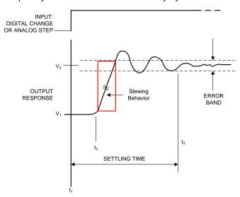
Figure 2. Large Signal Response of an Op-Amp
