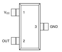
Figure 2. Pin Diagram (SOT-23 Package)
