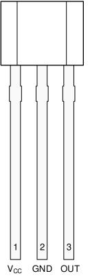
Figure 3. Pin Diagram (TO-92 Package)
