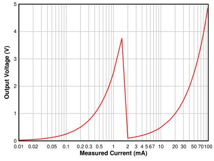
Figure 3-6. Output Voltage (V) Over Measurement Range, 10 µA to 100 mA, Log Scale
