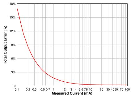
Figure 3-2. Total Output Error (%) Over Measurement Range,  $R_{SHUNT}$  = 1.984  $\Omega$ , 100  $\mu$ A to 100 mA, Ideal Shunt Tolerance
