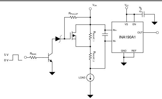
Figure 3-3. INA901 Schematic, 4 Decade Measurement
