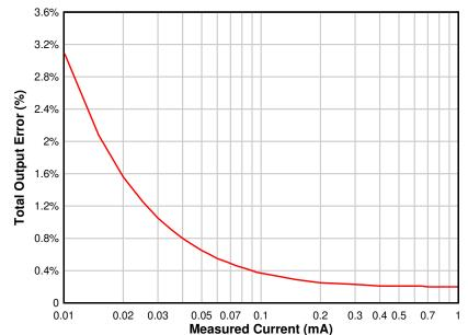
Figure 3-4. Total Output Error (%) Over Measurement Range,  $R_{SHUNT}$  = 100  $\Omega$ , 10  $\mu$ A to 1 mA, Ideal Shunt Tolerance
