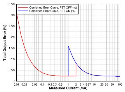
Figure 4-1. Total Output Error (%) Over Measurement Range, 10 µA to 100 mA, With Hysteresis
