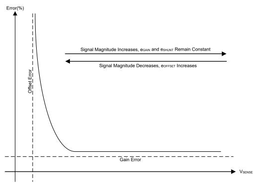
Figure 2-1. Current Sense Amplifier Error Curve Characteristics
