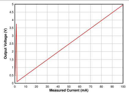
Figure 3-5. Output Voltage (V) Over Measurement Range, 10 µA to 100 mA
