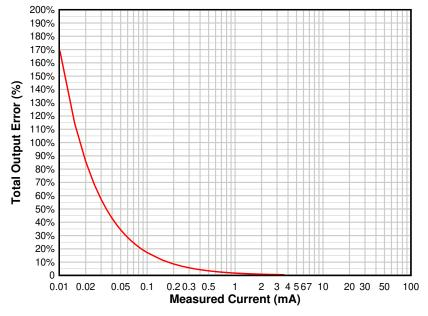
Figure 3-1. Total Output Error (%) Over Measurement Range,  $R_{SHUNT}$  = 1.984  $\Omega$ , 10  $\mu$ A to 100 mA, Ideal Shunt Tolerance
