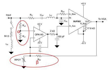
Figure 7.  $\alpha$  and  $\beta$  Resistor Network
