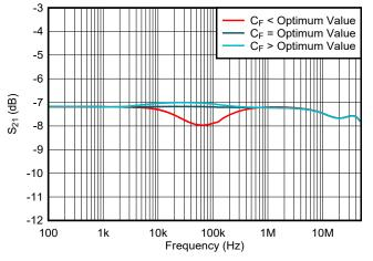
Figure 8. Tuning Output Response with Different C<sub>F</sub> Value
