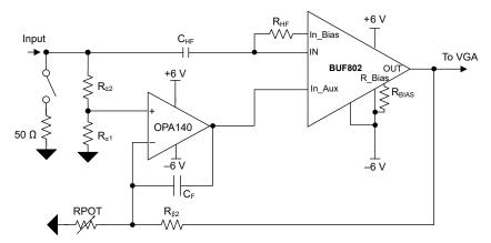
Figure 1. Generic Composite Loop Front-End Stage with OPA140 and BUF802
