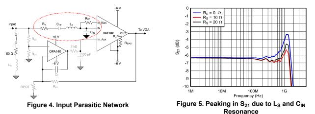
The peaking due to the resonance between  $L_S$  and  $C_{IN}$  can be dampened by the insertion of a series dampening resistor  $R_S$  as shown in Figure 4. Besides helping in dampening  $S_{21}$  peaking,  $R_S$  also helps with improvement of  $S_{11}$ . The exact math behind improvement of  $S_{11}$  is discussed in *Tuning of the*  $S_{11}$  *Parameter*.
