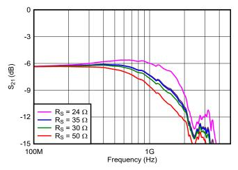
Figure 6. S<sub>21</sub> Input Response with Varying R<sub>S</sub>
