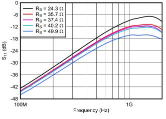
Figure 11. S<sub>11</sub> with Varying R<sub>S</sub>
