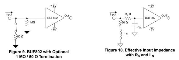
While it is possible to mount an exact 50- $\Omega$  termination to achieve the resistance at the input of the front-end composite loop circuit, the parasitic capacitance of the BUF802 (C<sub>IN</sub>) appears in parallel with the 50- $\Omega$  resistance resulting in a non-ideal termination across frequency.
