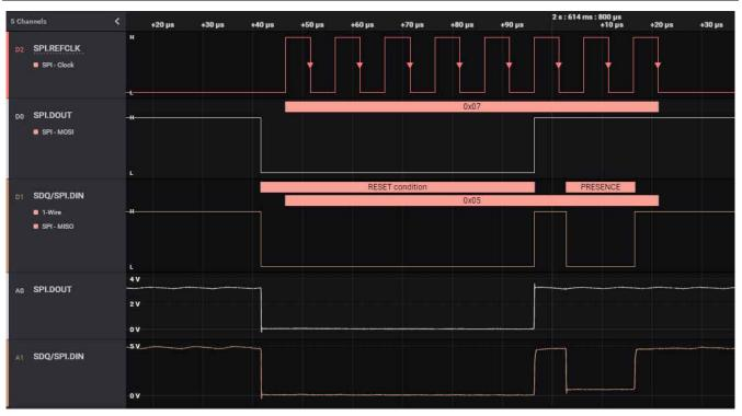
Figure 2-15. Scope Capture of Bus Reset and Response
