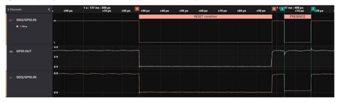
Figure 2-3. Scope Capture of Bus Reset and Response
