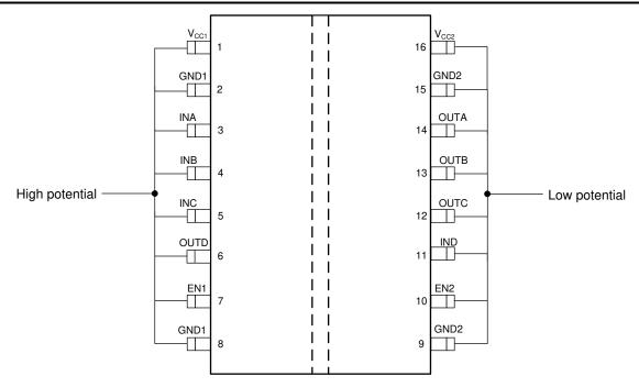
Figure 3-3. ISOS141-SEP SEDR Bias Diagram
