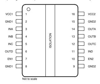
Figure 3-1. ISOS141-SEP Pinout Diagram
