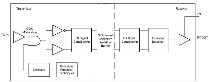
Figure 2-1. Functional Block Diagram of the ISOS141-SEP
