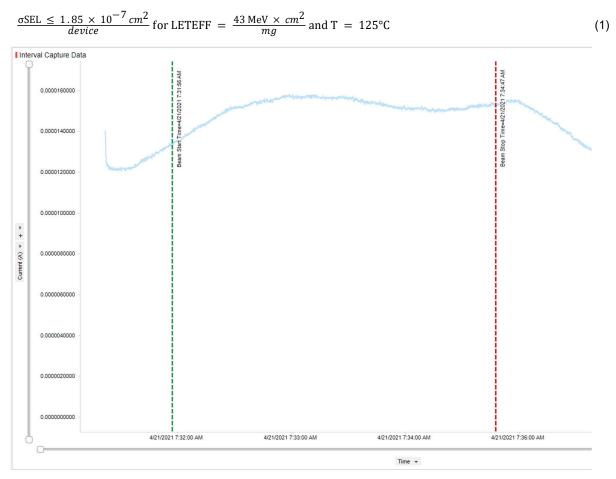
Figure 5-1. Current vs Time (I vs t) Data for Vs Current During SEL Run # 1
