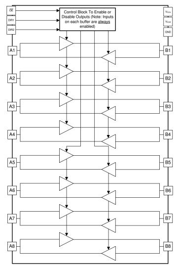
Figure 2-1. Functional Block Diagram of the SN54SLC8T245-SEP
