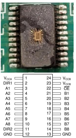
Figure 3-1. SN54SLC8T245-SEP Photograph and Pinout Diagram
