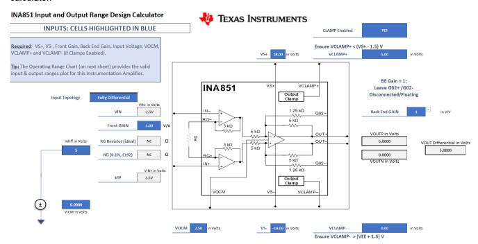
Figure 3. INA851 Input and Output Range Design Calculator
