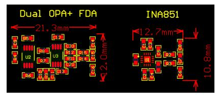
Figure 4. PCB Size Comparison
