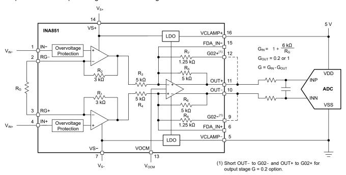
Figure 1. INA851 ADC Driver Application
