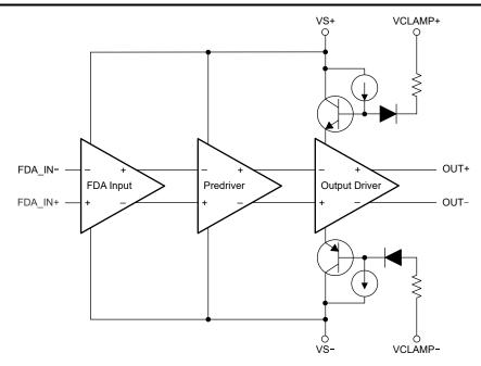
Figure 2. Simplified Schematic of Output Driver Clamping Structure
