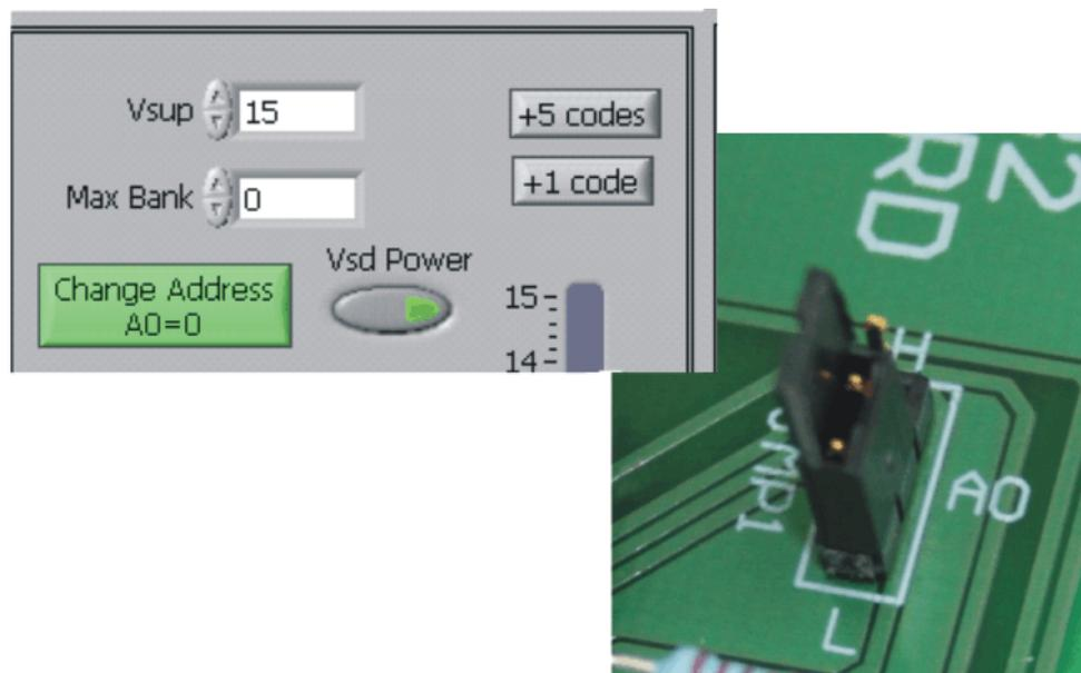
**Figure 15. BUF08832\_Test\_Board Jumper JMP1 Set For Logic '0'**
