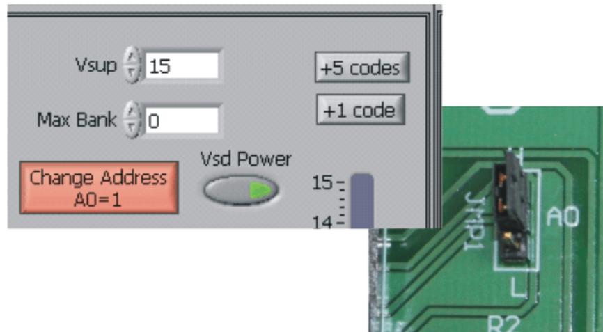
**Figure 14. BUF08832\_Test\_Board Jumper JMP1 Set For Logic '1'**
