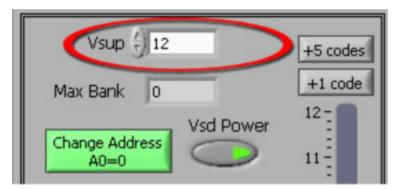
Figure 17. Measuring and Entering Power-Supply Voltage
