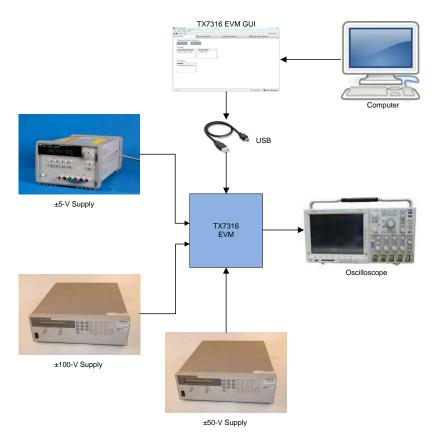
Figure 3. On-chip Beamforming Setup
