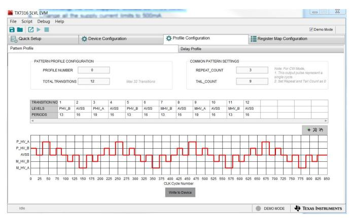
Figure 33. Profile Configuration - Pattern Profile
