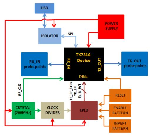
Figure 51. EVM Hardware Block Diagram
