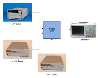
Figure 2. Off-chip Beamforming Setup
