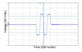
Frequency = 5 MHz; Peak to peak = 196.6 mV, Rise Time = 20.8 ns; Fall Time = 20.8 ns
