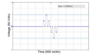
Frequency = 1.08 MHz; Peak-to-Peak = 196.5 mV Figure 5. Output Pattern When Switch S2 is Pressed
