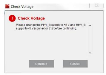
Figure 12. Pop-up Warning Given by the GUI When the CW Mode is Selected
