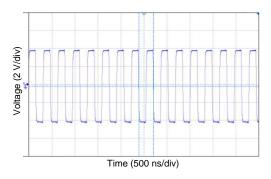
Frequency = 3.125 MHz; Peak-to-Peak = 8.08 V Figure 13. CW-Mode Output of the Device
