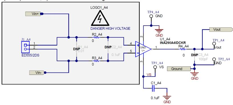
Figure 4. INA290EVM Schematic: Gain A4 Panel
