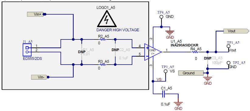
Figure 5. INA290EVM Schematic: Gain A5 Panel
