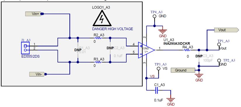
Figure 3. INA290EVM Schematic: Gain A3 Panel
