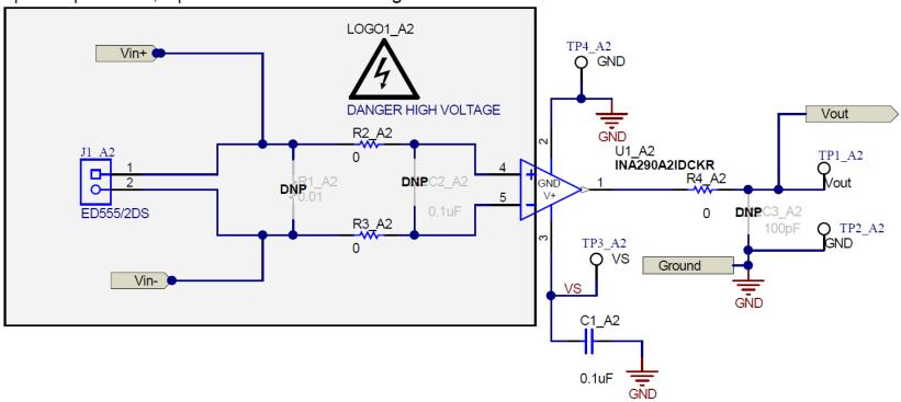
Figure 2. INA290EVM Schematic: Gain A2 Panel
