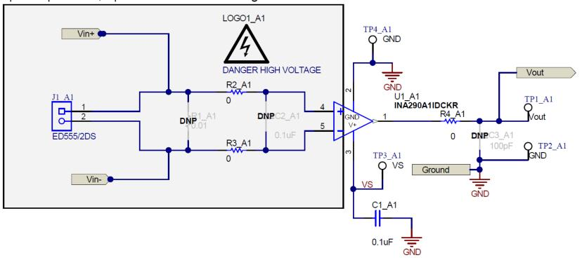
Figure 1. INA290EVM Schematic: Gain A1 Panel
