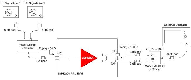
Figure 12. OIP3 Test Setup
