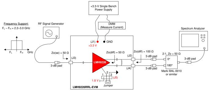
Figure 1. Single Tone Setup for Gain and Output P1dB
