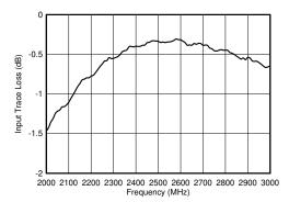
Figure 9. Input PCB Trace Loss vs Frequency
