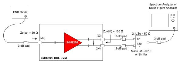
Figure 11. Noise Figure Test Setup
