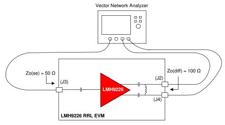
Figure 8. S-Parameter Test Setup
