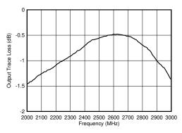
Figure 10. Output PCB Trace Loss vs Frequency
