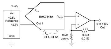
Figure 6. Single Supply 0V to +10V
