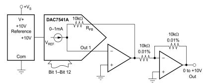
Figure 5. Another 0V to +10V Output DAC
