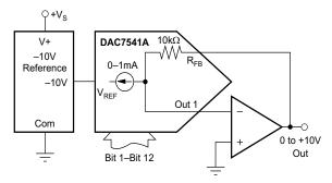
Figure 4. Precision 0V to +10V Output DAC
