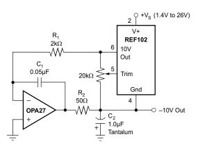
Figure 3. Improved –10V Reference with Improved Filter, with VOUT Trim
