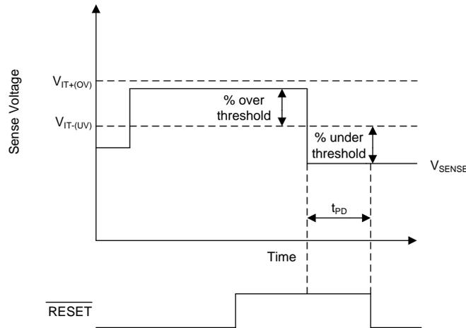
Figure 9. Measuring the Overdrive Voltage Curve
