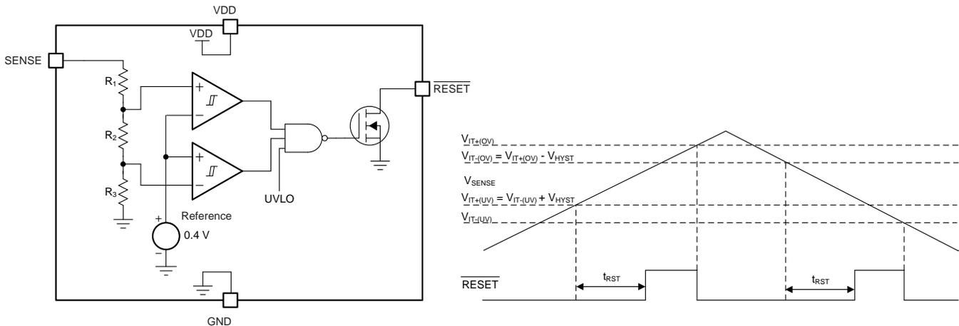
Figure 2. Window Supervisor Block Diagram and Timing Diagram
