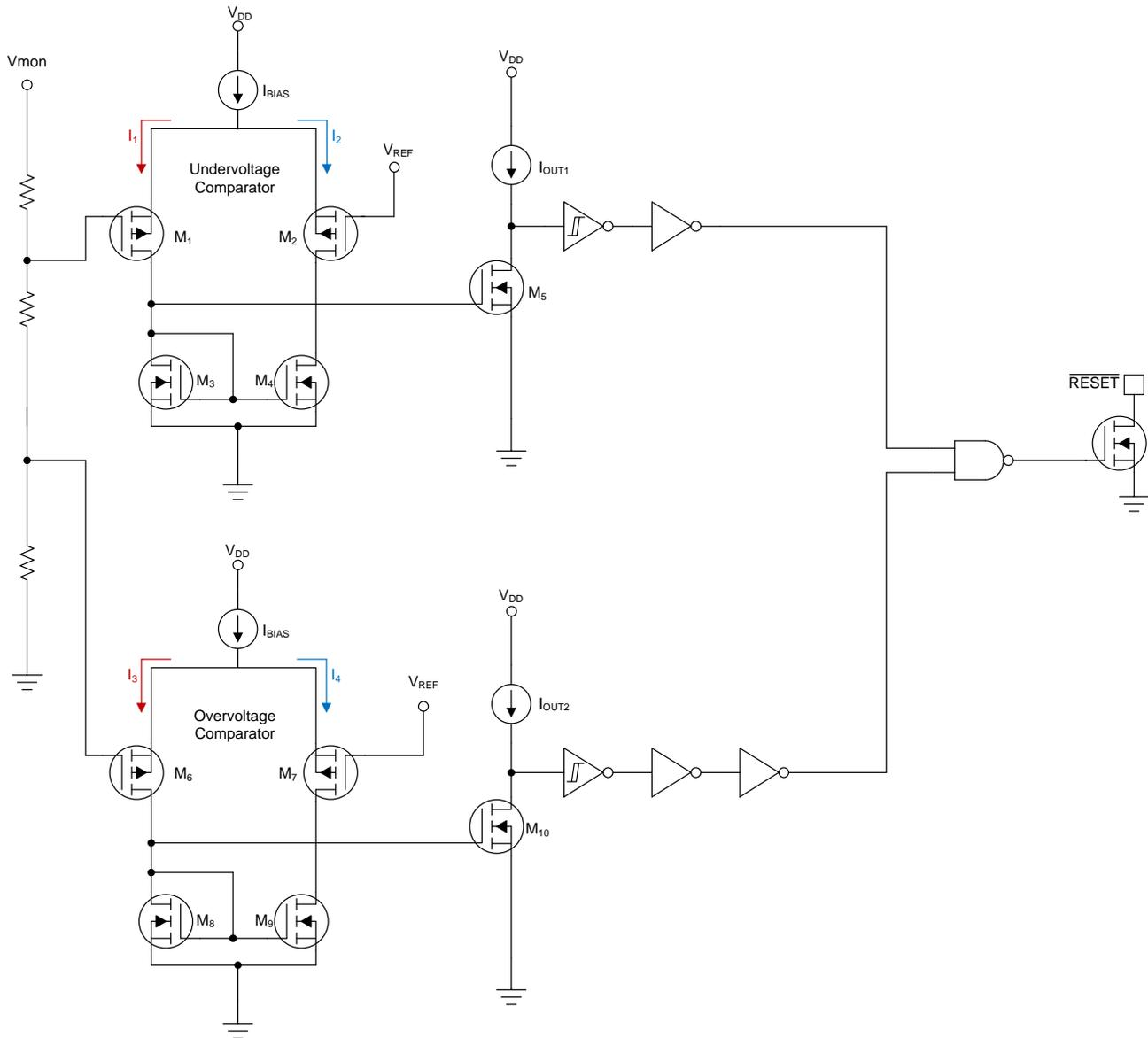
Figure 5. Window Supervisor Architecture With a Single Output
