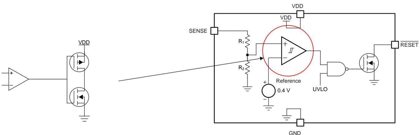
Figure 4. Comparator with Push-Pull Output
