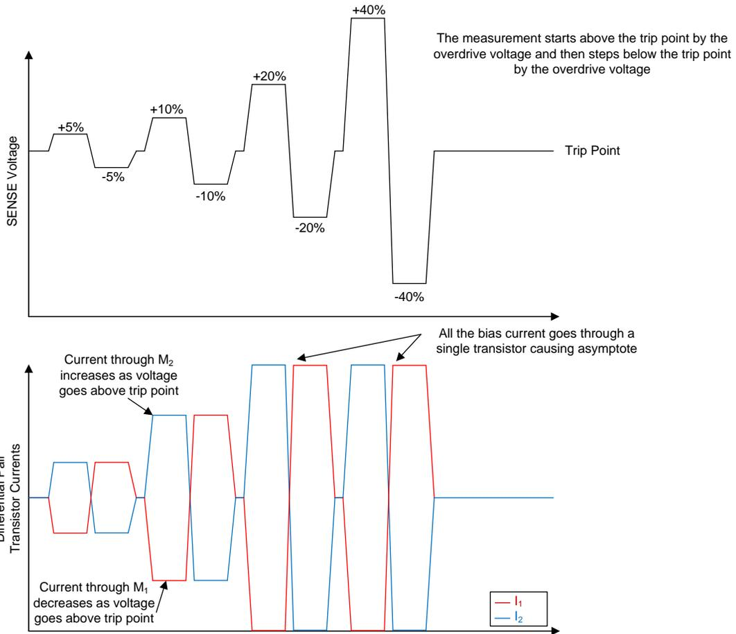
Figure 10. Current in Differential Pair for How Overdrive Voltage is Measured
