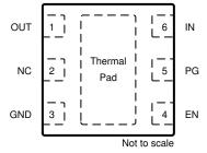
Figure 4-1. Pin Diagram Adjustable TPS745-Q1 DRV Package
