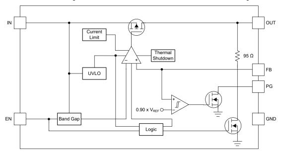
Figure 1-1. Adjustable Version With Open-Drain Power-Good
