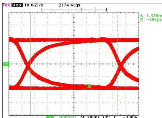
Figure 3. Eye Pattern Diagram at 700 Mbps, PRBS Pattern of  $2^7-1$
