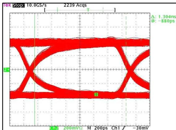
Figure 4. Eye Pattern Diagram at 700 Mbps, PRBS Pattern of  $2^{23}-1$
