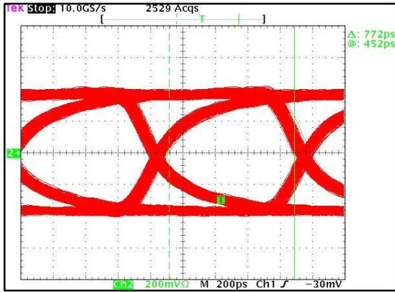
Figure 7. Eye Pattern Diagram at 1.1 Gbps, PRBS Pattern of  $2^7-1$
