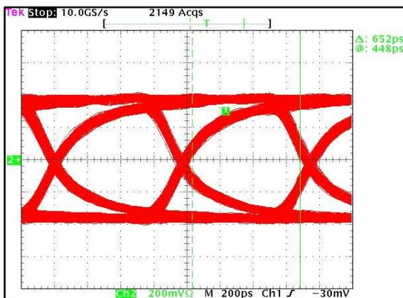
Figure 9. Eye Pattern Diagram at 1.3 Gbps, PRBS Pattern of  $2^7-1$
