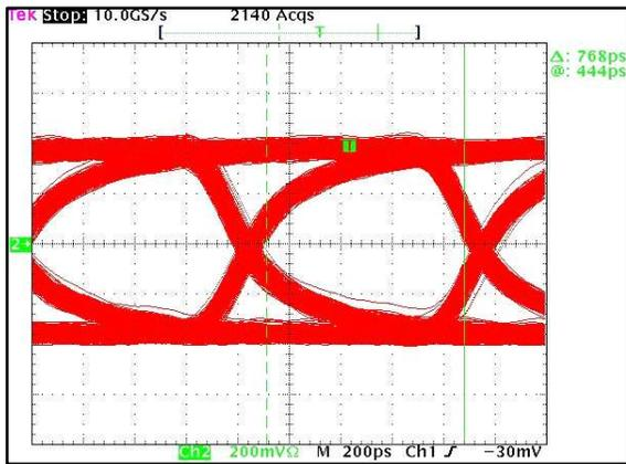
Figure 8. Eye Pattern Diagram at 1.1 Gbps, PRBS Pattern of  $2^{23}-1$
