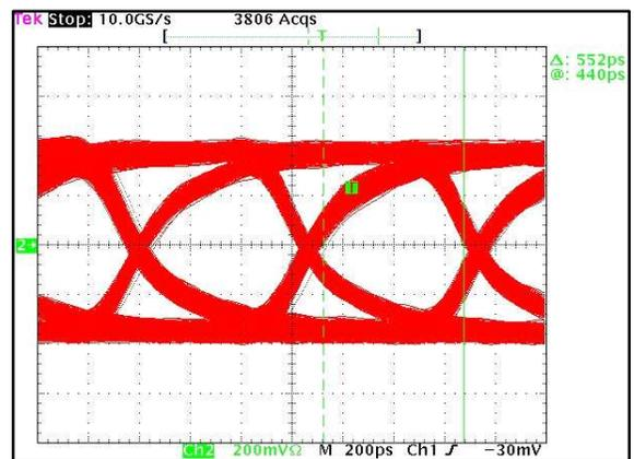
Figure 12. Eye Pattern Diagram at 1.5 Gbps, PRBS Pattern of  $2^{23}-1$
