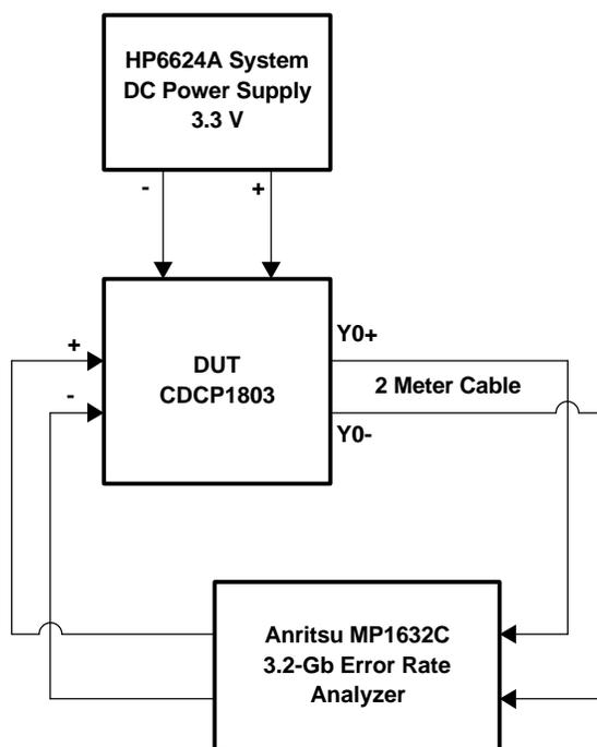
Figure 1. Test Setup for BER Measurements
