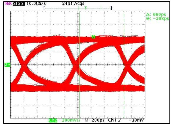
Figure 10. Eye Pattern Diagram at 1.3 Gbps, PRBS Pattern of  $2^{23}-1$
