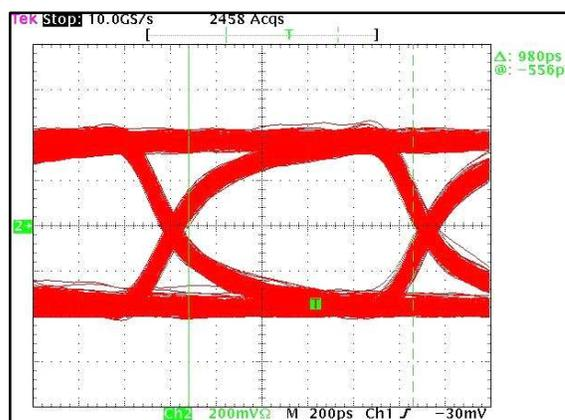
Figure 6. Eye Pattern Diagram at 900 Mbps, PRBS Pattern of  $2^{23}-1$
