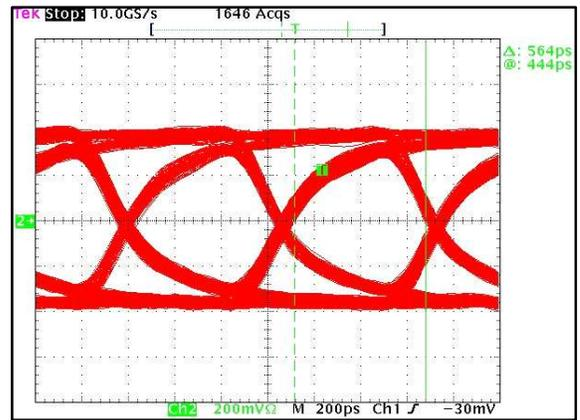
Figure 11. Eye Pattern Diagram at 1.5 Gbps, PRBS Pattern of  $2^7-1$
