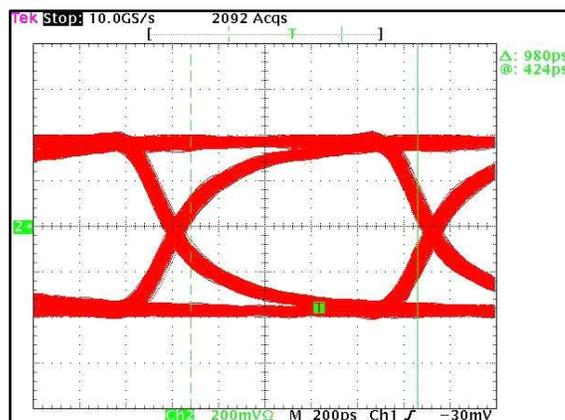
Figure 5. Eye Pattern Diagram at 900 Mbps, PRBS Pattern of  $2^7-1$
