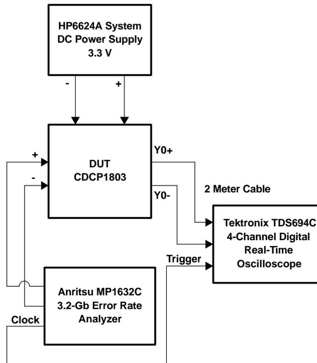
**Figure 2. Test Setup for Eye Diagrams**
