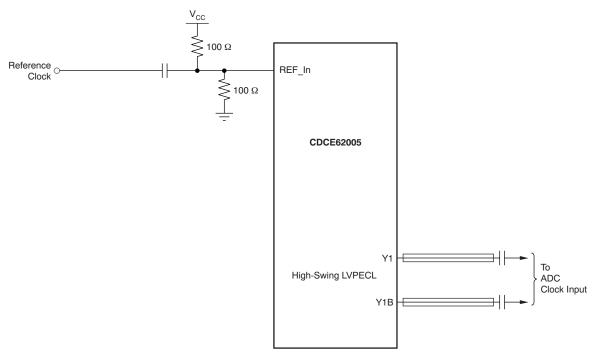
Figure 8. CDCE62005 Interface to ADCs for Low IF Input Frequencies
