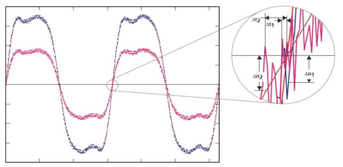
Figure 6. Thermal Noise Effect for Different Slope Clock Signals
