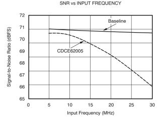
Figure 12. SNR Performance vs IF Input Frequency
