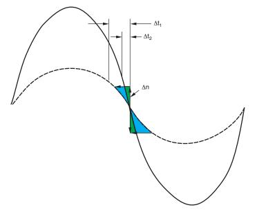
Figure 7. Thermal Noise Effect for Different Amplitude Sinusoids
