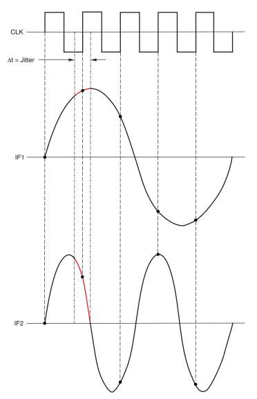
Figure 3. SNR Degradation Caused by Jitter for Different IF Input Signals
