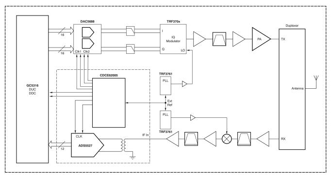
Figure 1. ADS5527 with CDCE62005 Clocking Solution within a Typical Base Station Application
