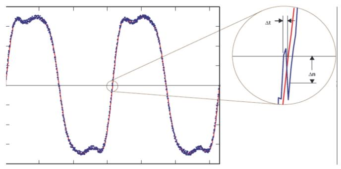
Figure 5. Sampling Error Caused by Thermal Noise Component
