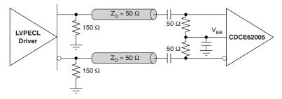
Figure 13. LVPECL AC-Coupled Termination Circuit
