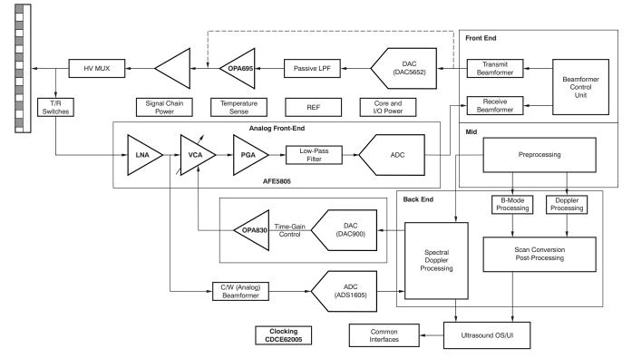
Figure 20. Typical Medical Ultrasound System Clocking Solution
