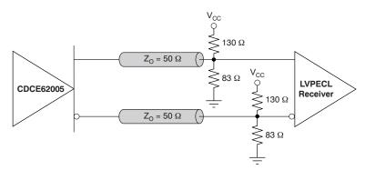
Figure 7. LVPECL DC Termination Circuit
