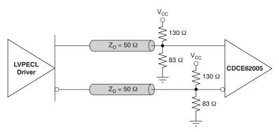
Figure 12. LVPECL DC Termination Circuit
