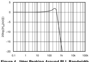
Figure 4. Jitter Peaking Around PLL Bandwidth
