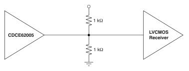
Figure 11. 3.3-V LVCMOS DC-Coupled Termination Circuit
