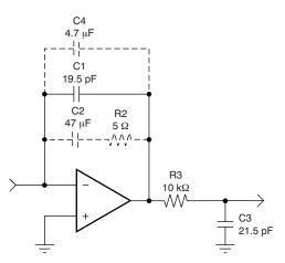
Note: Components shown with a dashed line are off-chip.
