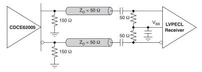
Figure 8. LVPECL AC-Coupled Termination Circuit
