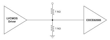
Figure 16. 3.3-V LVCMOS DC-Coupled Termination Circuit
