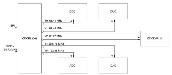
Figure 19. Typical Wireless Basestation System Clocking Solution
