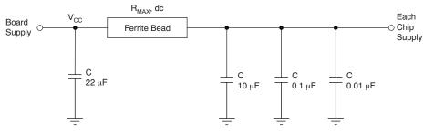
Figure 18. Power-Supply Decoupling
