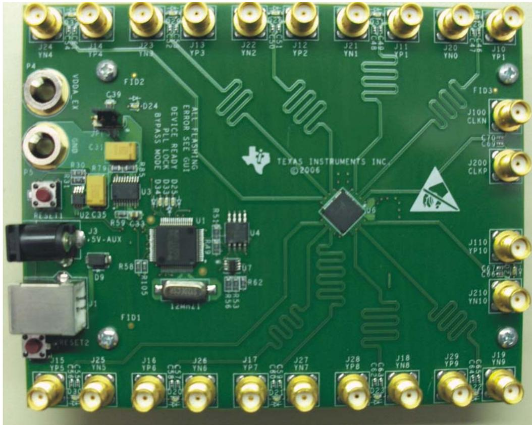
**Figure 1. CDCL6010 Evaluation Board**
