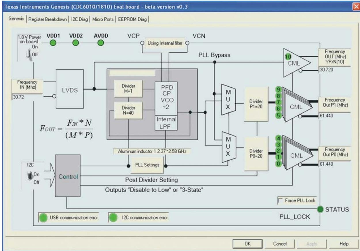
Figure 7. TI Genesis Software GUI
