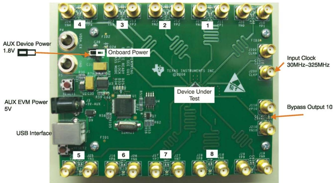
Figure 2. CDCL6010EVM Controls and Connectors
