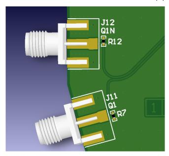
Figure 6. On Board Optional Output Termination
