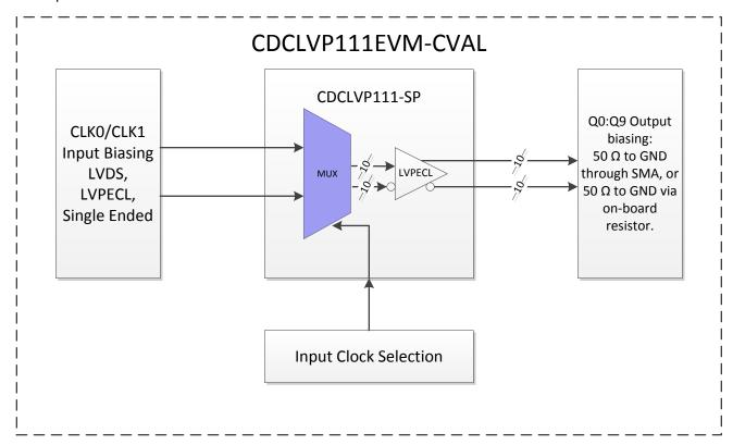
Figure 1. CDCLVP111-SP EVM Block Diagram
