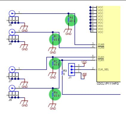
Figure 3. Input Biasing Schematic
