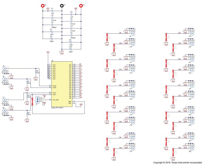
Figure 7. CDCLVP111-SP Schematic
