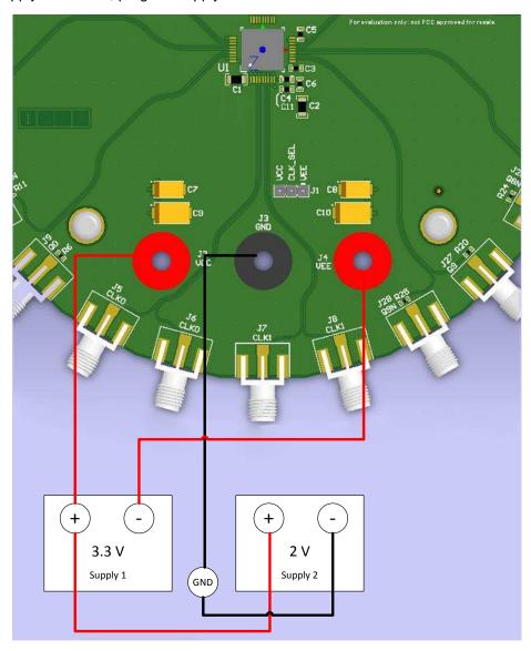
**Figure 2. Power Supply Connections**
