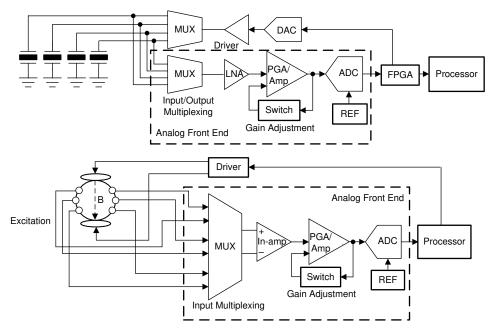
Figure 2. Analog Front-End Implementation for Ultrasonic and Magnetic Flowmeter
