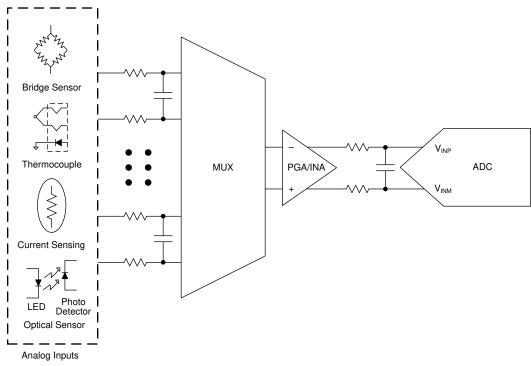
Figure 3. Multiplexed Analog Input Front End
