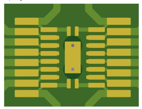
Figure 1-3. TSSOP (PW)-SOT-23-Thin (DYY)-WQFN (BQB)
