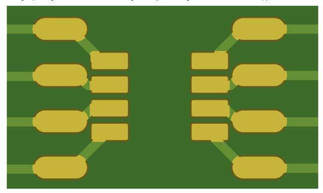
Figure 1-1. Example of a SOT-23 (DCN) Footprint Within a SOIC (D) Footprint
