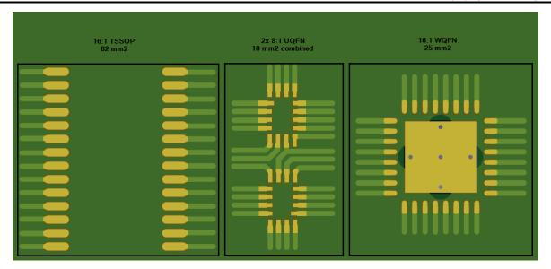
Figure 1-6. PCB Space Savings Using Two 8:1 Devices Instead of One 16:1 Device
