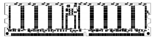
Figure 6. One Side of DIMM With SDRAMs, PLL, and SPD Mounted
