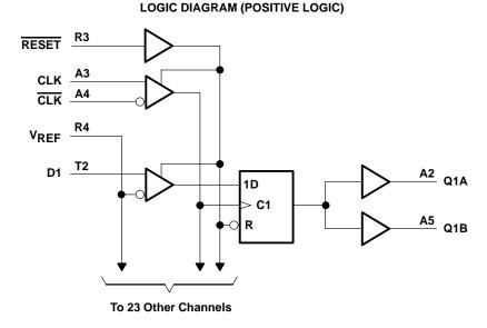
Figure 4. Function Table and Logic Diagram of SN74SSTV32852
