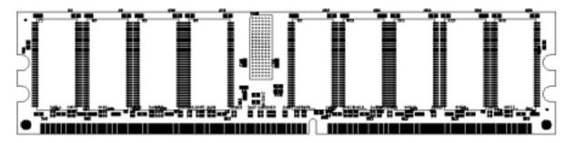
Figure 7. Other Side of DIMM With SN74SSTV32852 Mounted
