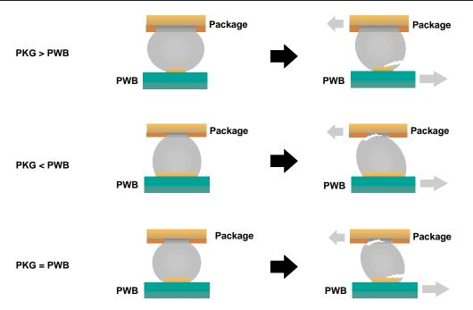
Figure 13. Solder-Ball Behavior During Thermal Cycling
