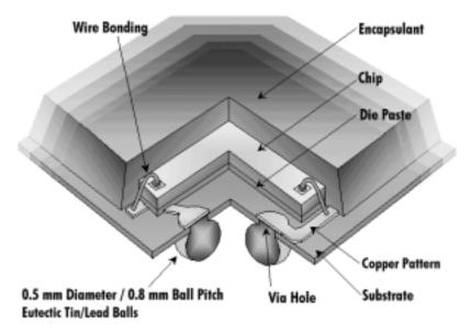
Figure 11 shows the construction of the 114-ball LFBGA package.
