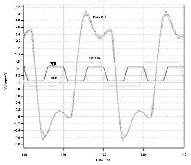
Figure 9. Simulation Results of SN74SSTV32852 Into a Raw-Card C Load
