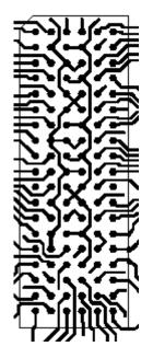
Figure 8. Example Routing of SN74SSTV32852 Register
