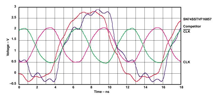
Figure 7. Q2 Output Switching In-Phase (Synchronously) With Ten Other Outputs
