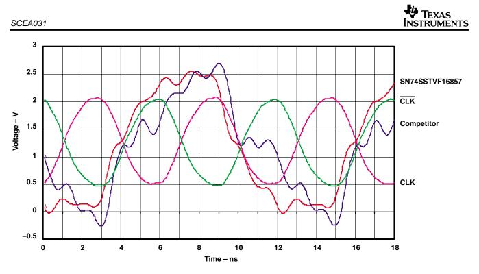
Figure 8. Q2 Output Switching Out-of-Phase (Complementarily) with Ten Other Outputs
