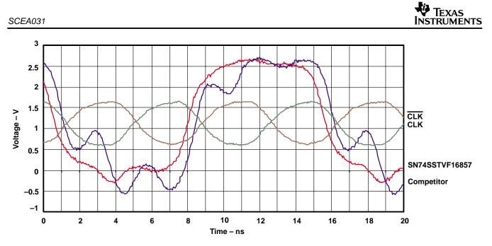
Figure 6. Single-Bit (Q2 Output) Switching Results on Raw Card Version B RDIMM
