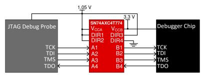
Figure 2-10. JTAG Voltage Translation Using SN74AXC4T774
