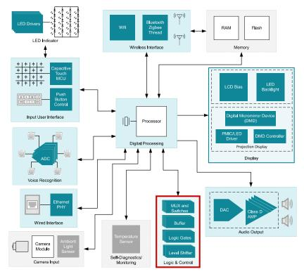
Figure 2-4. Smart Speaker and Smart Display
