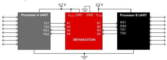
Figure 2-7. Two 2-wire UART Interface Voltage Translation Using SN74AXC4T245
