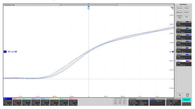
Figure 2-14. 104 ps Channel-to-Channel Skew for SN74AXC8T245
