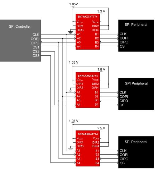
Figure 2-2. SPI Interface Using SN74AXC4T774 Device
