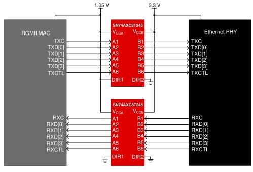
Figure 2-12. RGMII Voltage Translation Using SN74AXC8T245
