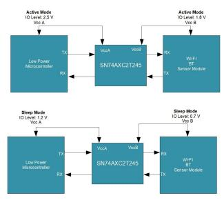
Figure 2. Low-Voltage Translation Use Case Between MCU and Wireless Peripheral
