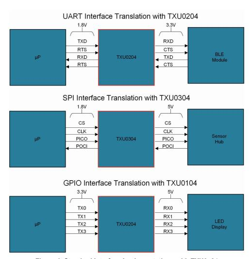
Figure 1. Standard Interface Implementations with TXU0x04
