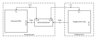
Figure 1. Example of Level Translation With an Enhanced FPGA
