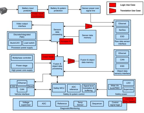
Figure 1. Simplified Block Diagram for ADAS Domain Controller
