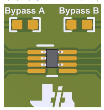
Figure 2. 5-pin DCK Placement
