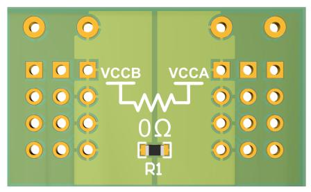
Figure 3. Single Supply Configuration
