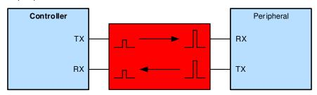
Figure 3-1. Example 2-wire UART Voltage Translation Block Diagram
