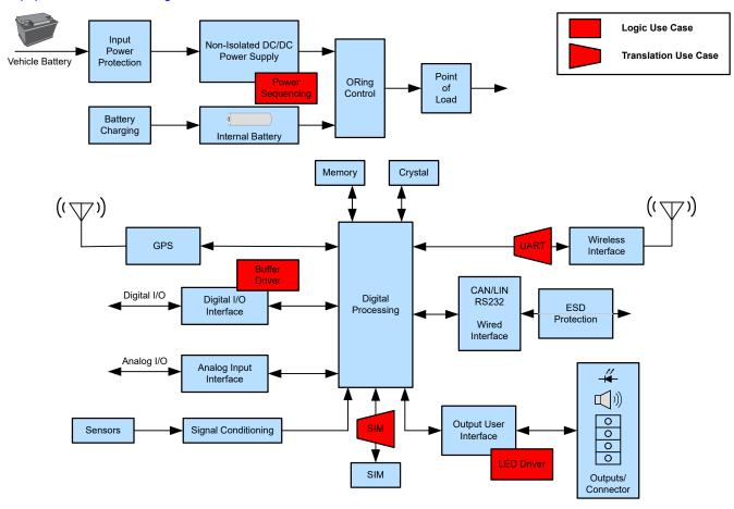
Figure 1-1. Simplified Block Diagram for Asset Trackers
