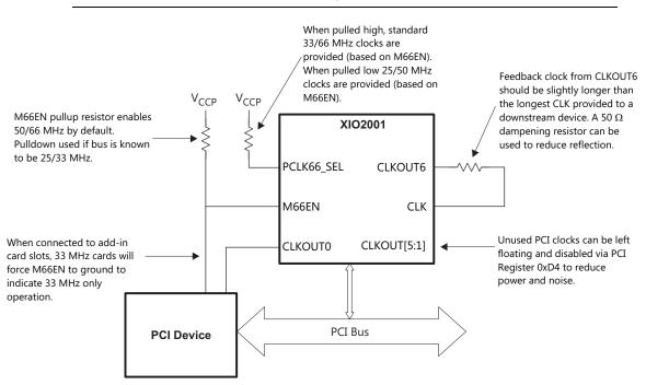
Figure 3. External PCI Bus Clock Configuration
