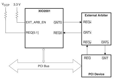
**Figure 4. External Arbiter Connections**
