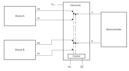
Figure 5. TMUX154E Application Diagram
