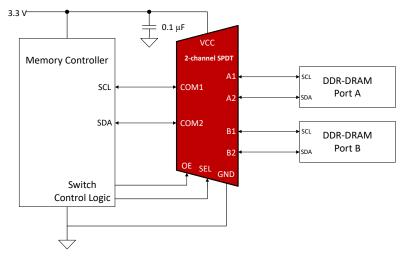
Figure 3. I3C DDR-DRAM Switch Example
