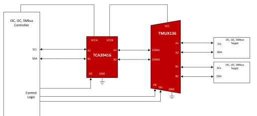
Figure 7. Flexible 2:1 I3C Bus with Signal Boost - TMUX136 + TCA39416
