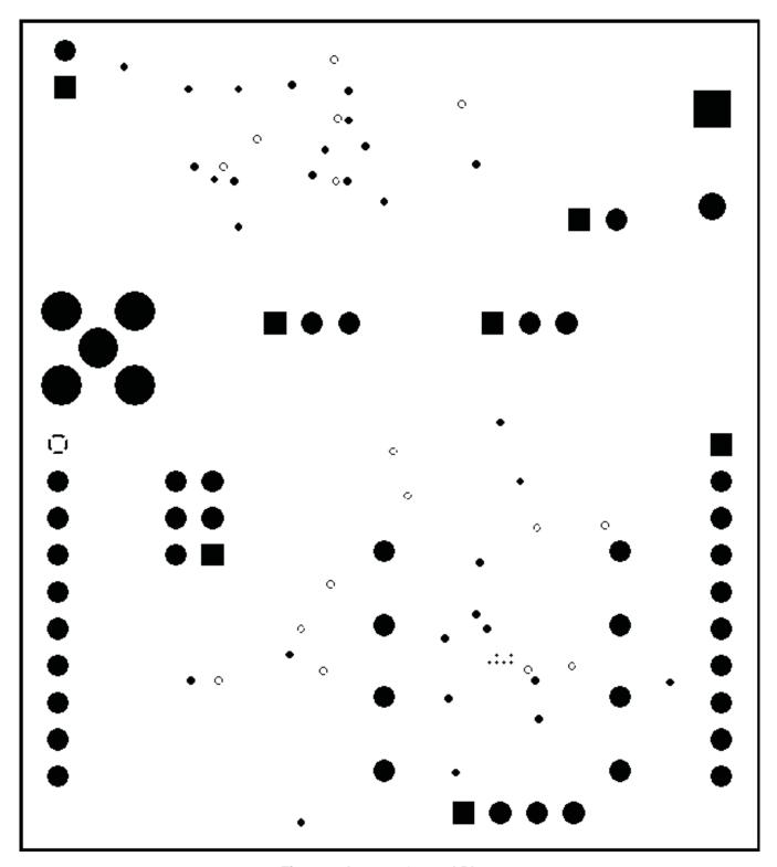
Figure 7. Layer 3 Ground Plane
