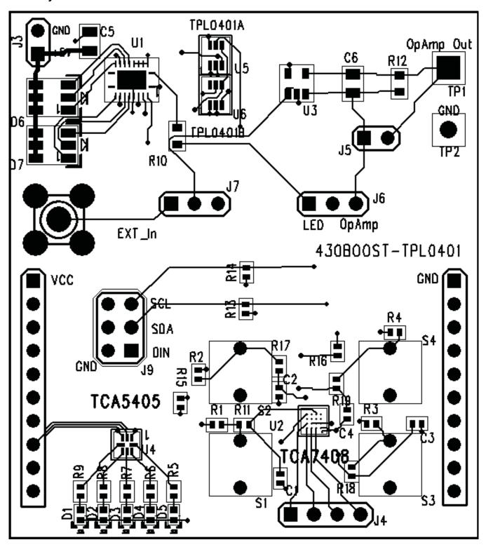
Figure 5. Routing, Assembly and Silkscreen Top
