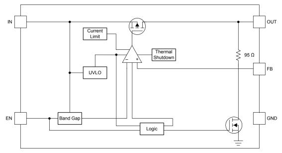
Figure 1-1. TLV759P Functional Block Diagram
