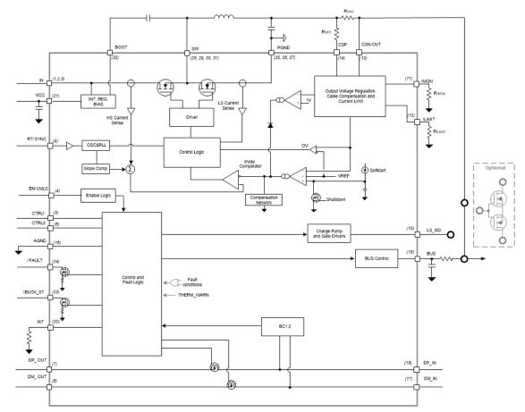
Figure 1-1. Functional Block Diagram
