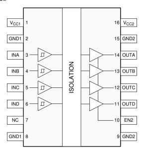
Figure 4-1. Pin Diagram (16-DW) Package
