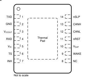
Figure 4-2. Pin Diagram (TCAN11625-Q1 DMT Package)
