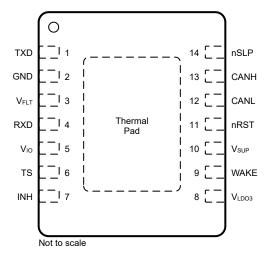
Figure 4-1. Pin Diagram (TCAN11623-Q1 DMT) Package
