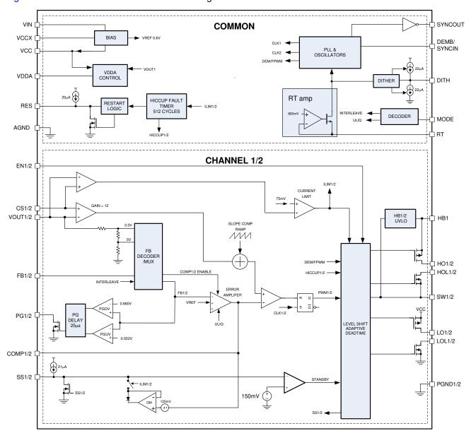
Figure 1-1. Functional Block Diagram
