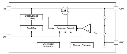
Figure 1-1. Functional Block Diagram
