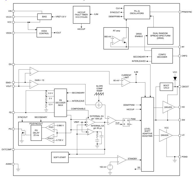
Figure 1-1. Functional Block Diagram
