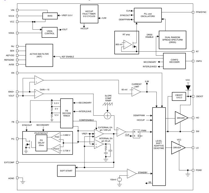
Figure 1-1. Functional Block Diagram
