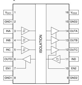
Figure 4-1. Pin Diagram (common for 16-QSOP Packages)
