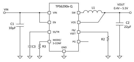
Figure 3-3. Selectable V<sub>O</sub> Operation Schematic
