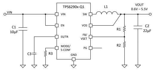
Figure 3-2. Adjustable V<sub>O</sub> Operation Schematic
