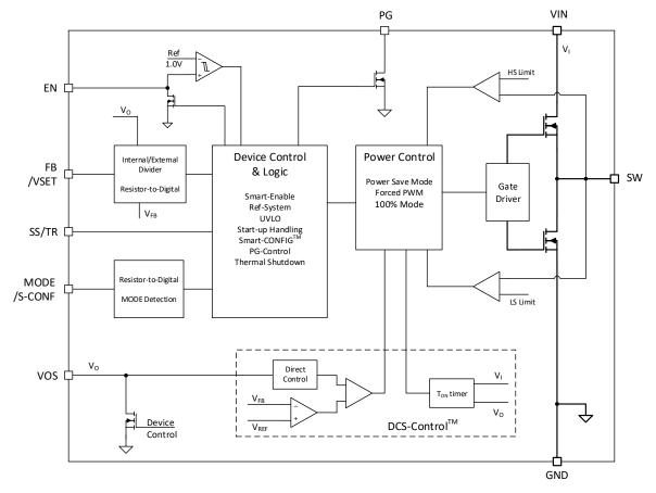
Figure 1-1. Functional Block Diagram
